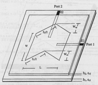
Figure 5. The geometry of the dual port compact microstrip antenna.
