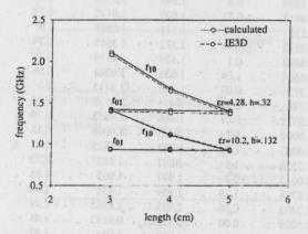
**Figure 6.** The variation of the  $TM_{10}$  and  $TM_{01}$  mode frequencies with the length *L* for different dielectric constant ( $e_r$ ) and thickness (*h*) values for the dual port antenna (W = 5 cm,  $W_{cd} = 1$  cm,  $W_{cp} = 1$  cm).
