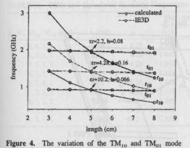
frequencies with the length L for different dielectric constant ( $\varepsilon_r$ ) and thickness (*h*) values ( $W = 5 \text{ cm}, W_{cp} = 1 \text{ cm},$
