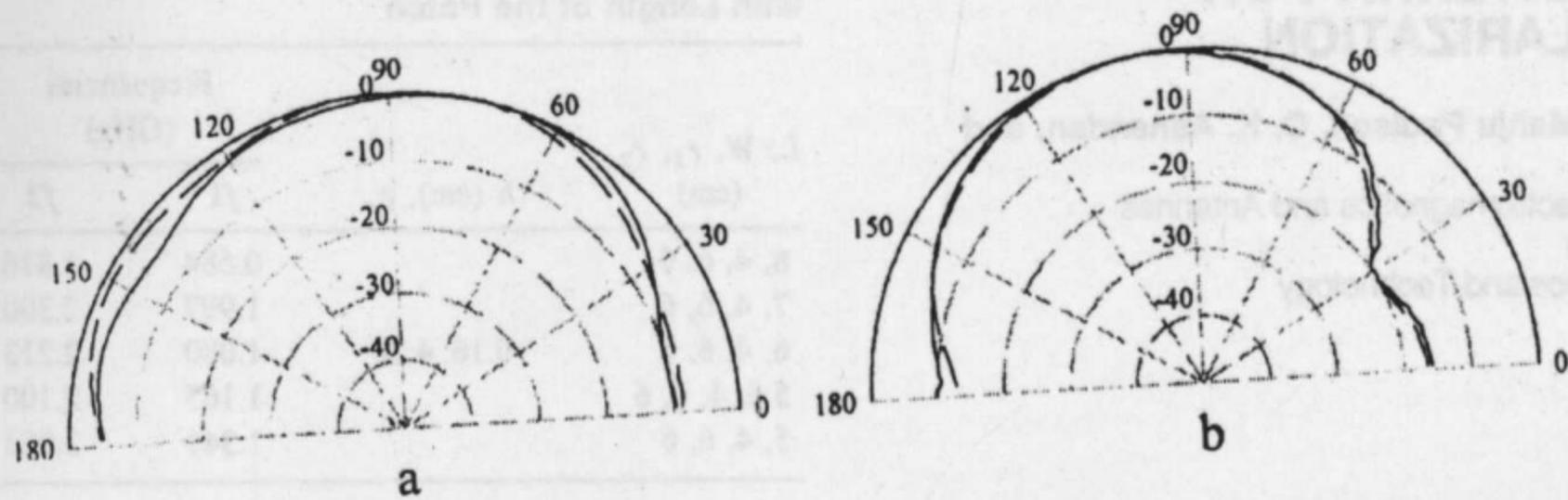
Figure 4 Radiation patterns for 1.885 GHz. (a) *E* plane, (b) *H* plane. Solid lines, copolar; dashed lines, cross polar
