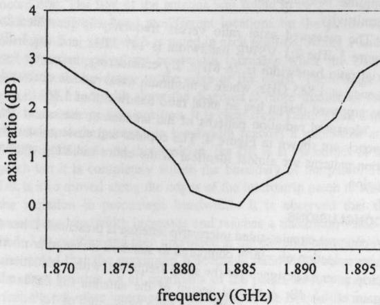
**Figure 3** Measured axial ratio against frequency
