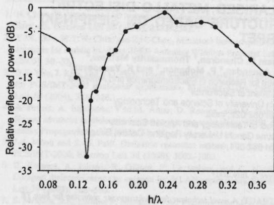
**Figure 6** Variation of relative reflected power with dielectric thickness at stage 3
