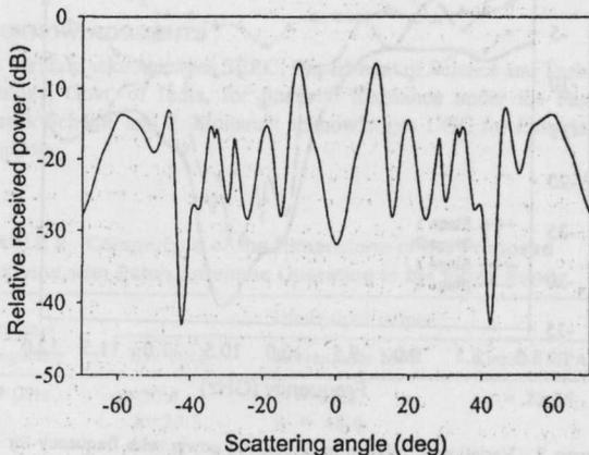
**Figure 5** Variation of relative received power with scattering angle at stage 3 with  $h = 3.91$  mm and  $f = 10.5$  GHz
