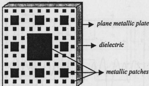
**Figure 2** Schematic diagram of the reflector-backed metallo-dielectric structure of the third iterated stage
