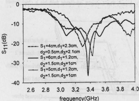
**Figure 2** Variation of  $S_{11}$  with frequency for different feed lengths of the antenna ( $h_1 = h_2 = 0.16$  cm,  $\epsilon_{r1} = \epsilon_{r2} = 4.28$ ,  $L = 4$  cm,  $W = 2$  cm,  $S_2 = 3.5$  cm)
