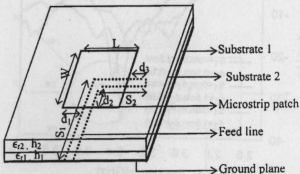
Figure 1 Geometry of the planar L-strip-fed microstrip antenna
