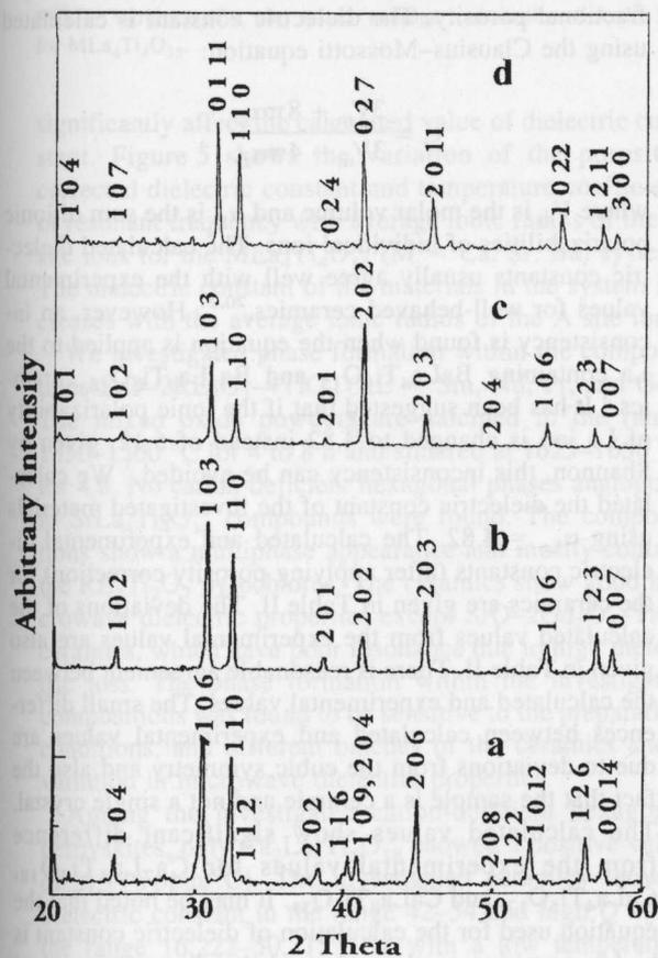
FIG. 1. X-ray diffraction patterns of (a) BaLa<sub>4</sub>Ti<sub>4</sub>O<sub>15</sub>, (b) SrLa<sub>4</sub>Ti<sub>4</sub>O<sub>15</sub>, (c) CaLa<sub>4</sub>Ti<sub>4</sub>O<sub>15</sub>, and (d) Ca<sub>2</sub>La<sub>4</sub>Ti<sub>5</sub>O<sub>18</sub>.
