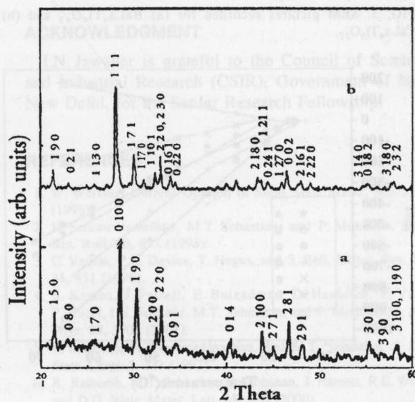
FIG. 2. X-ray diffraction patterns of (a) CaLa<sub>4</sub>Ti<sub>5</sub>O<sub>17</sub> and (b) CaLa<sub>8</sub>Ti<sub>9</sub>O<sub>31</sub>.
