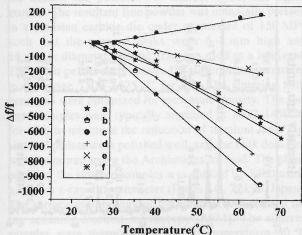
FIG. 4. Plot of  $\Delta f/f$  against temperature (a) SrLa<sub>4</sub>Ti<sub>4</sub>O<sub>15</sub>, (b) CaLa<sub>4</sub>Ti<sub>4</sub>O<sub>15</sub>, (c) Ca<sub>2</sub>La<sub>4</sub>Ti<sub>5</sub>O<sub>18</sub>, (d) Ca<sub>2</sub>La<sub>4</sub>Ti<sub>5</sub>O<sub>17</sub>, and (e) CaLa<sub>8</sub>Ti<sub>9</sub>O<sub>31</sub>.
