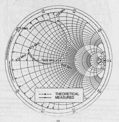
Fig. 7. Theoretical and experimental impedance loci of the antennas A, B, and C. (a) Antenna A.
