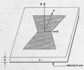
Fig. 1. Geometry of the proposed compact microstrip antenna with coordinate system.
