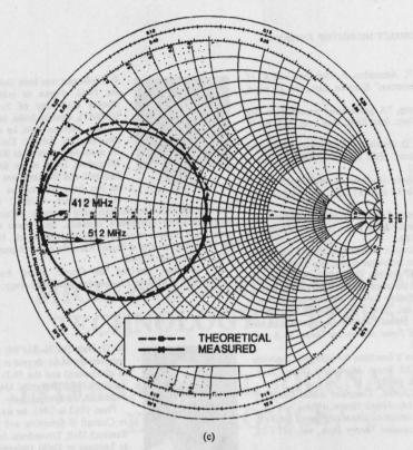
Fig. 7. (Continued.) Theoretical and experimental impedance loci of the antennas A, B, and C. (c) Antenna C.
