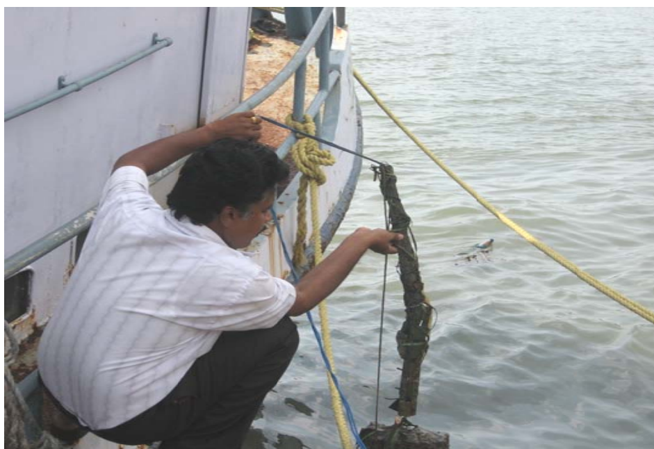
Fig. 2.6 Brass panels retrieved after every exposure period
