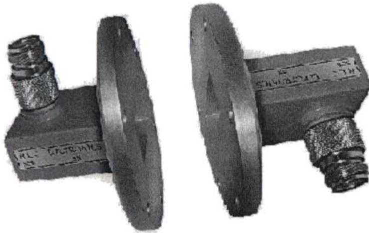
Figure 2.4 Coaxial to wave guide adapters to measure the S parameters.
