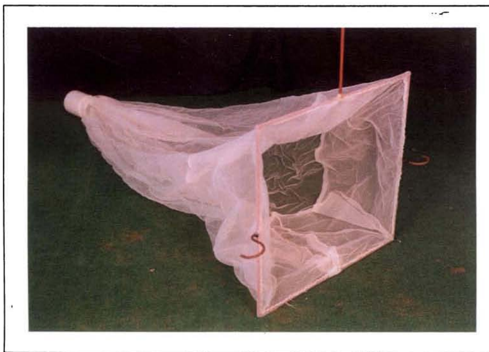
Fig 3.1 Sampling net used to collect migrating postlarvae.
