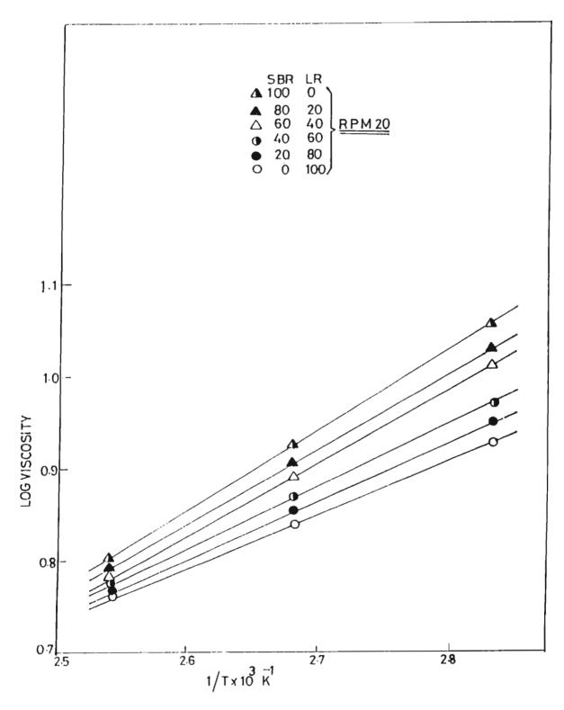
FIG.4.10: Variation in viscosity with temperature of SBR/LR blends at 20 rpm
