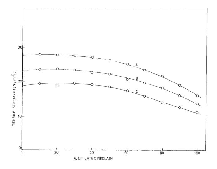
FIG.3.30: Variation in tensile strength with latex reclaim of NR/LR blends
