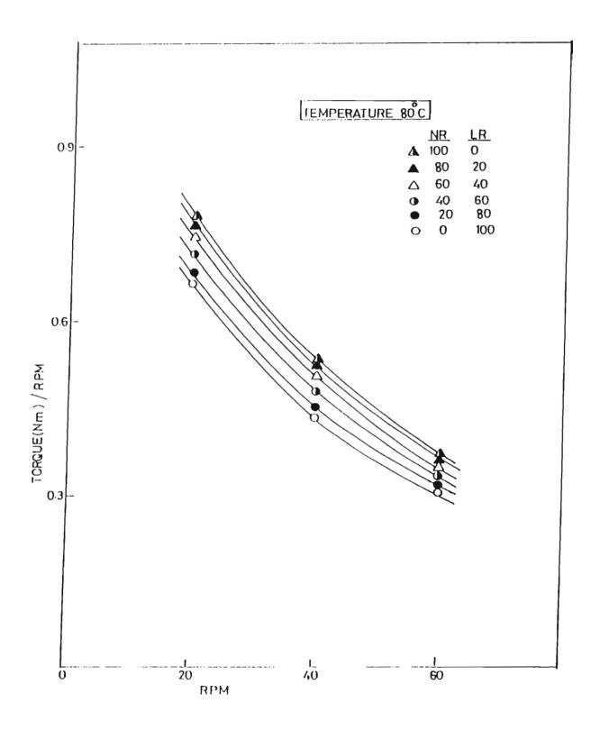
FIG.3.27: Variation in viscosity with shear rate of NR/LR blends at 80°C
