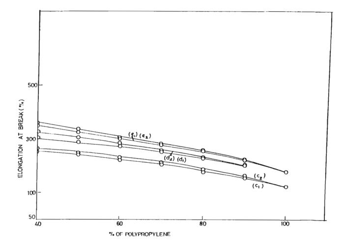
FIG.5.4: Variation in elongation at break with polypropylene of crosslinked  $c_1$ ,  $d_1$ ,  $e_1$  (PP/NR);  $c_2$ ,  $d_2$ ,  $e_2$  (PP/LR) blends
