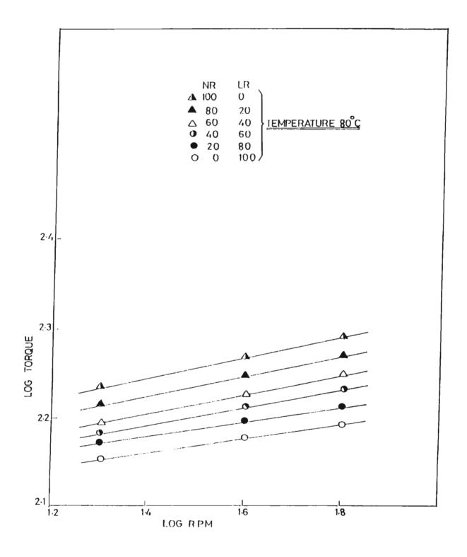
FIG.3.28: Variation in torque with shear rate of NR/LR blends at 80°C
