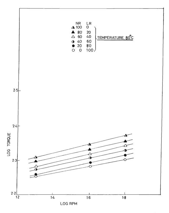
FIG.3.49: Variation in torgue with shear rate of NR/LR blends at 80°C
