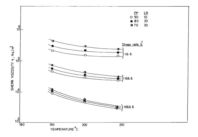
FIG.5.13: Variation in shear viscosity with temperature of PP/LR blends
