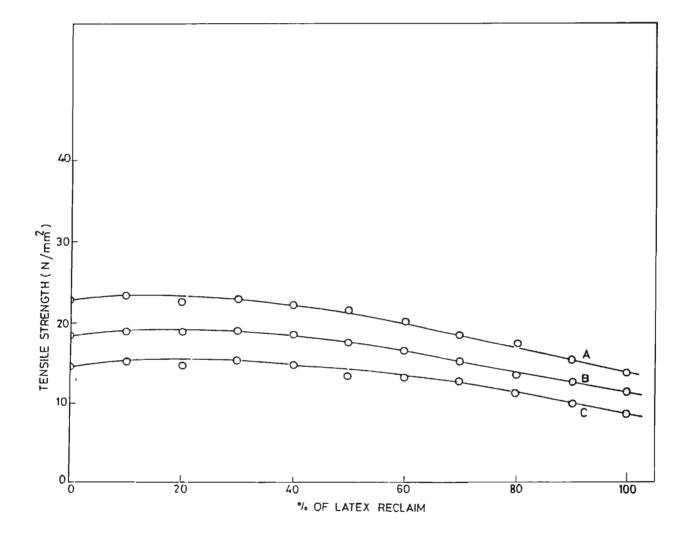
FIG.3.3: Variation in tensile strength with latex reclaim of NR/LR blends
