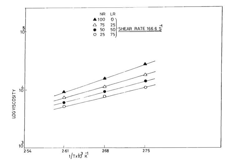
FIG.3.53: Variation in viscosity with temperature of NR/LR blends at a shear rate of 166.6  $\rm s^{-1}$
