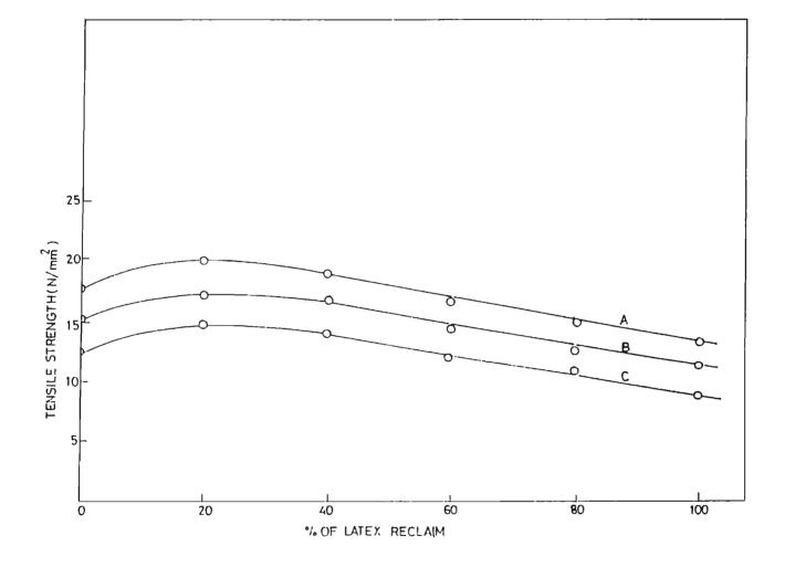
FIG.4.4: Variation in tensile strength with latex reclaim of SBR/LR blends
