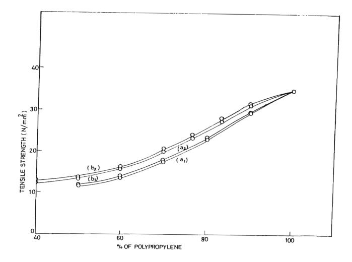
FIG.5.1: Variation in tensile strength with polypropylene of uncrosslinked a<sub>1</sub>, b<sub>1</sub> (PP/NR); a<sub>2</sub>, b<sub>2</sub> (PP/LR) blends
