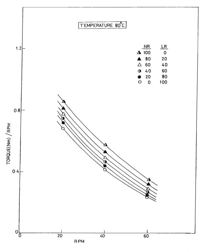
FIG.3.48: Variation in viscosity with shear rate of NR/LR blends at 80°C
