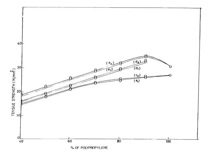
FIG.5.2: Variation in tensile strength with polypropylene of crosslinked c<sub>1</sub>, d<sub>1</sub>, e<sub>1</sub> (PP/NR); c<sub>2</sub>, d<sub>2</sub>, e<sub>2</sub> (PP/LR) blends
