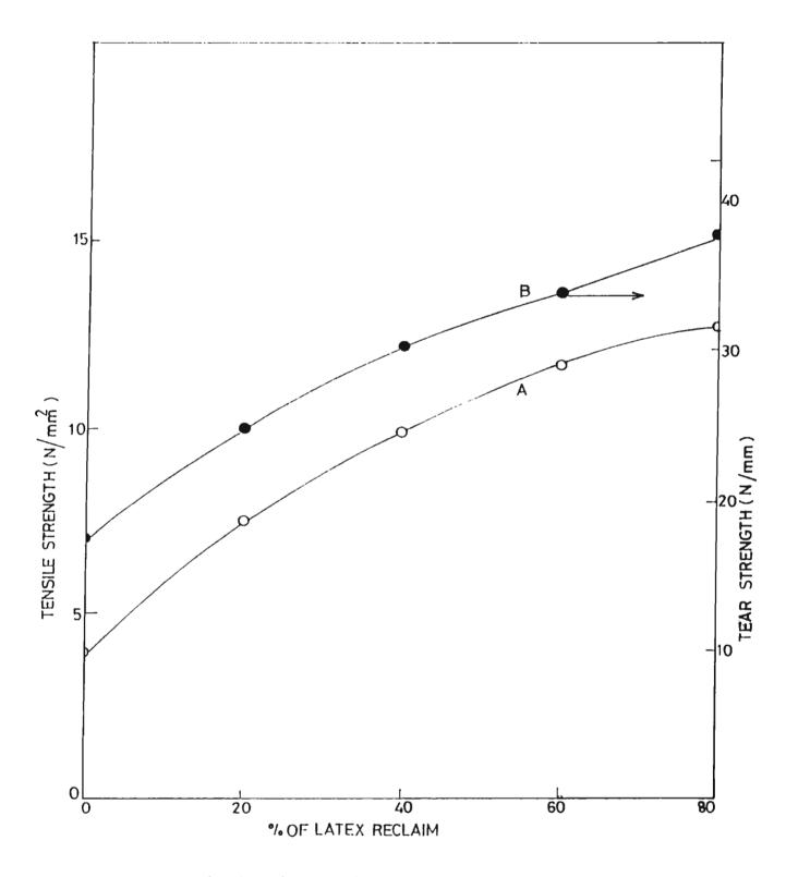
FIG.4.1: Variation in tensile strength and tear strength with latex reclaim of SBR/LR blends
