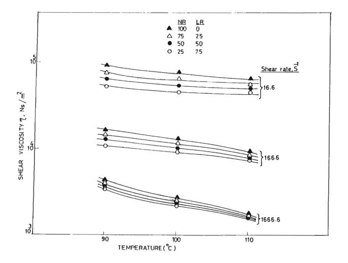
FIG.3.52: Variation in shear viscosity with temperature of NR/LR blends
