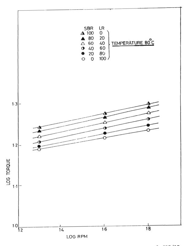
FIG.4.9: Variation in torque with shear rate of SBR/LR blends at 80°C
