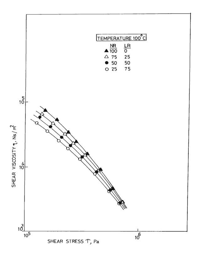
FIG.3.51: Variation in shear viscosity with shear stress of NR/LR blends at 100°C
