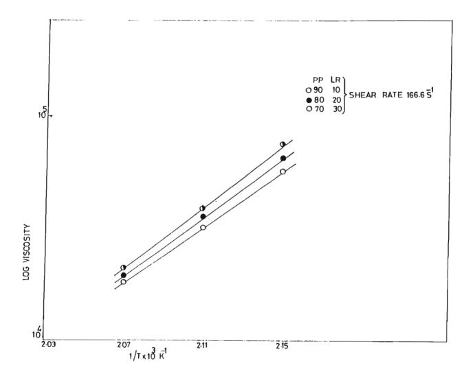
FIG.5.14: Variation in viscosity with temperature of PP/LR blends at a shear rate of 166.6  $s^{-1}$
