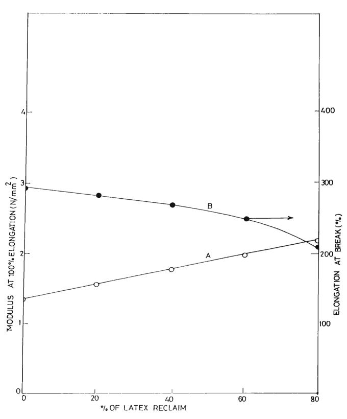
FIG.4.2: Variation in modulus and elongation at break with latex reclaim of SBR/LR blends
