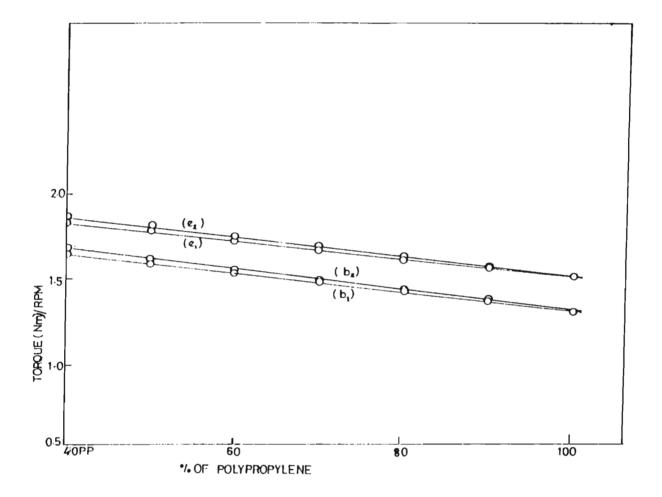
FIG.5.5: Variation in viscosity with polypropylene of uncrosslinked b<sub>1</sub> (PP/NR); b<sub>2</sub> (PP/LR) and crosslinked e<sub>1</sub> (PP/NR); e<sub>2</sub> (PP/LR) blends
