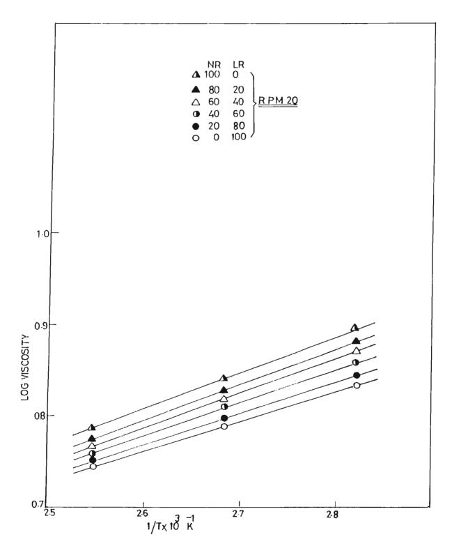
FIG.3.50: Variation in viscosity with temperature of NR/LR blends at 20 rpm
