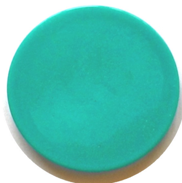
Figure 5.8 Photograph of 10% \text{La}_2\text{Cu}_{0.8}\text{Li}_{0.2}\text{Ge}_{1.8}\text{P}_{0.2}\text{O}_8 coated on PMMA.
