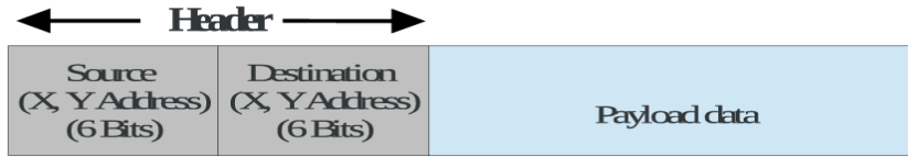
Figure 1.3 Flit format in an 8 x 8 mesh NoC
