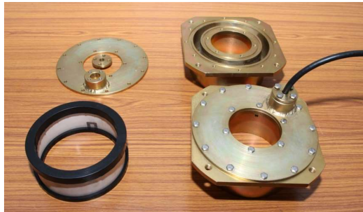
Fig. 4.22 Oil filled free-flooded transducer with steel housing.
