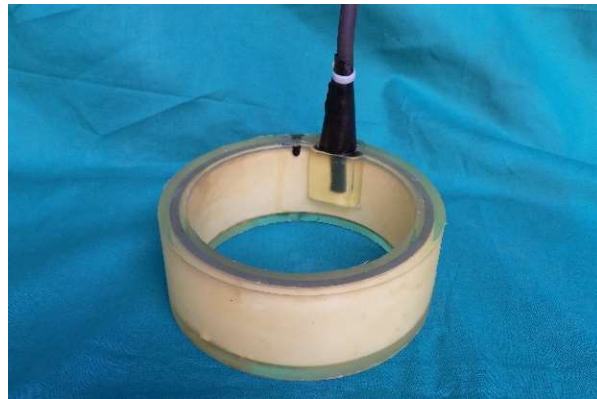
Fig. 4.20 PU moulded transducer.
