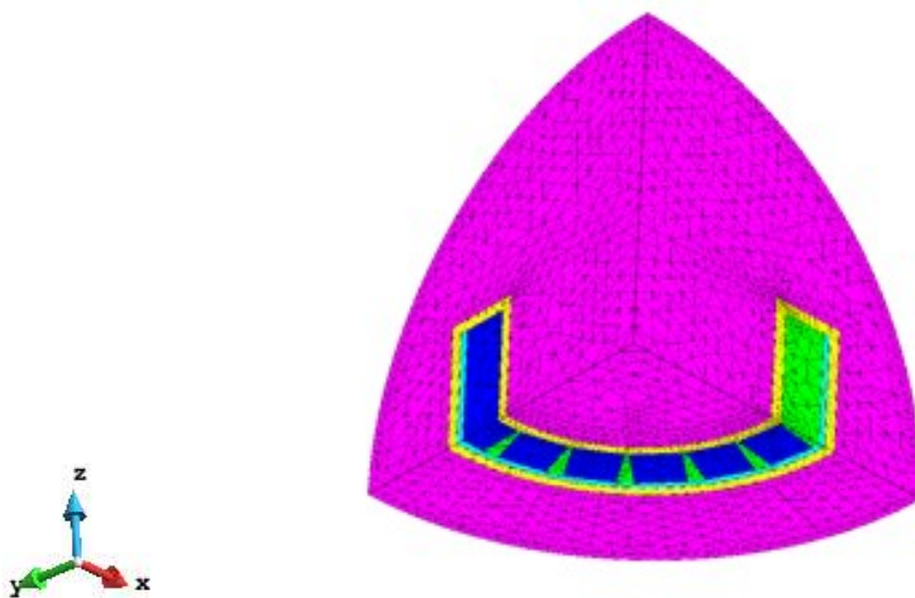
Fig. 4.58 3D model of the transducer in water.
