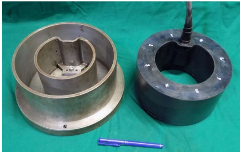
Fig. 5.11 Mould tool and PU moulded directional segmented ring transducer.
