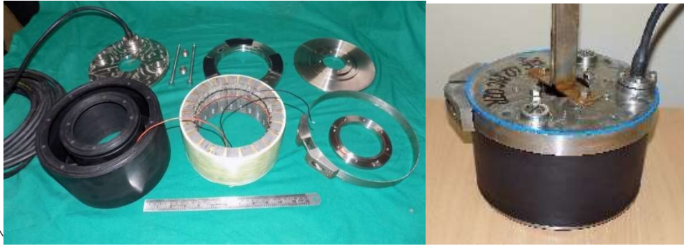
Fig. 4.70 Parts and fully assembled oil filled metal ceramic transducer.
