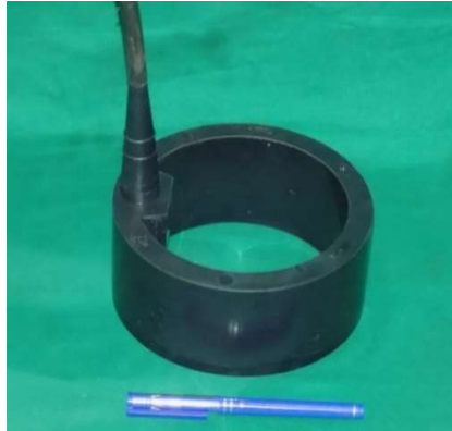
Fig. 5.6 PU moulded directional RPC transducer.
