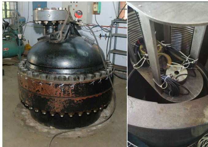
Fig. 4.35 Pressure testing of transducers.
