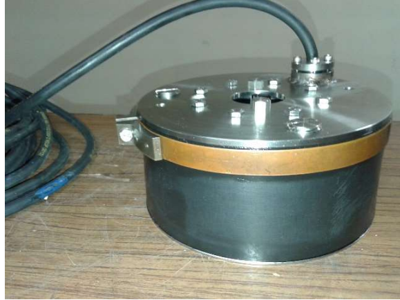
Fig. 4.21 RPC transducer with an oil filled rubber boot.
