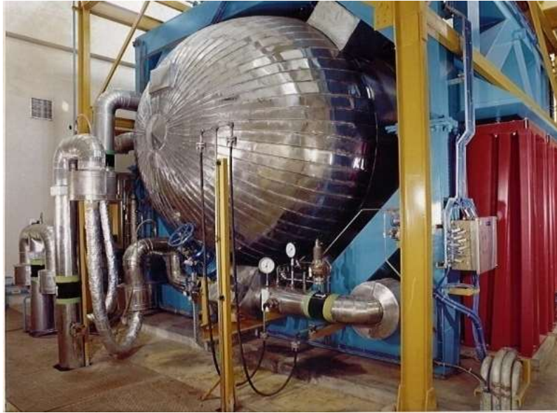
Fig. 4.25 Pressurised acoustic test chamber at NPOL.
