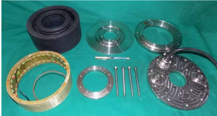
Fig. 4.48 Components of oil filled segmented ring transducer
