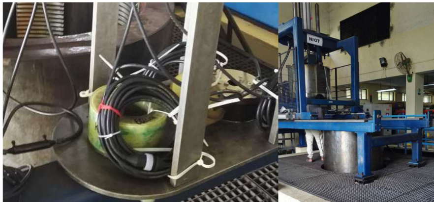
Fig. 4.81 Pressure test in the hyperbaric test facility.
