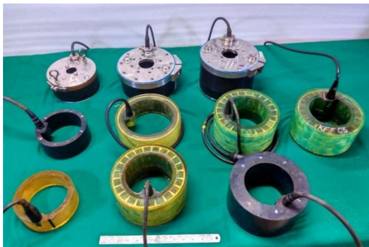
Fig. 6.1 Free-flooded ring transducer variants developed.
