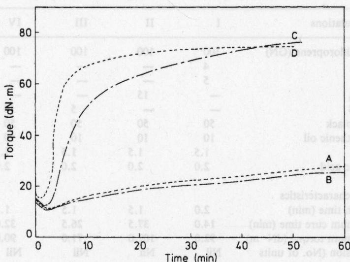
Fig. 1. Cure curves of W type CR. (A) MgO/ZnO, (B) TBLS, (C) MgO/ZnO + NA-22, (D) TBLS + NA-22.
