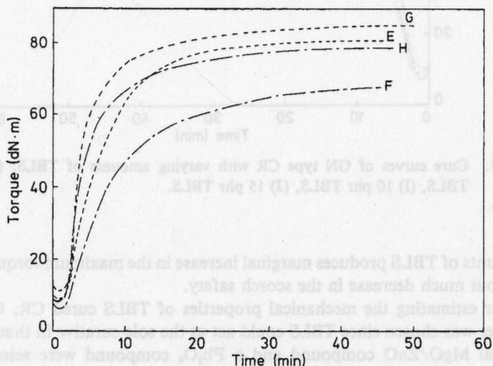
Fig. 2. Cure curves of GN type CR. (E) MgO/ZnO, (F) TBLS, (G) MgO/ZnO + NA-22, (H) TBLS + NA-22.
