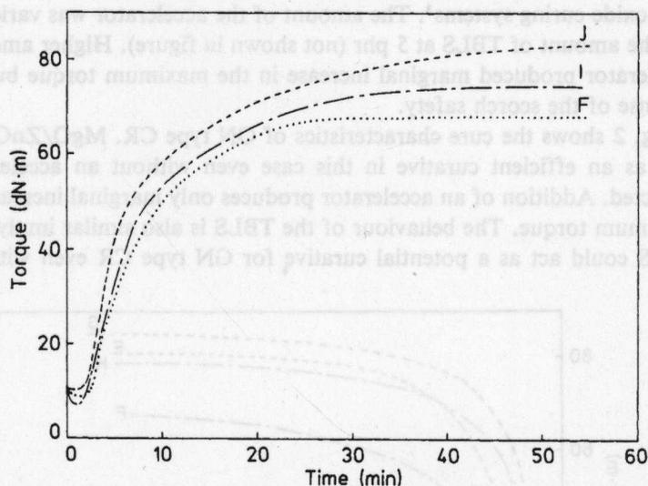
Fig. 3. Cure curves of GN type CR with varying amounts of TBLS: (F) 5 phr TBLS, (I) 10 phr TBLS, (J) 15 phr TBLS.
