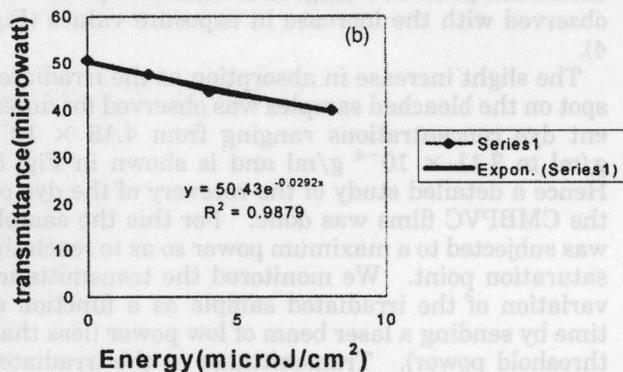
Fig. 6. (a) Recovery of the dye on CMBPVC film after irradiation [plot of energy  $\text{mJ}/\text{cm}^2$  versus transmittance (mW)]. (b) Exponential behavior of the recovery of the sample [plot of energy  $\text{mJ}/\text{cm}^2$  versus transmittance (mW)].
