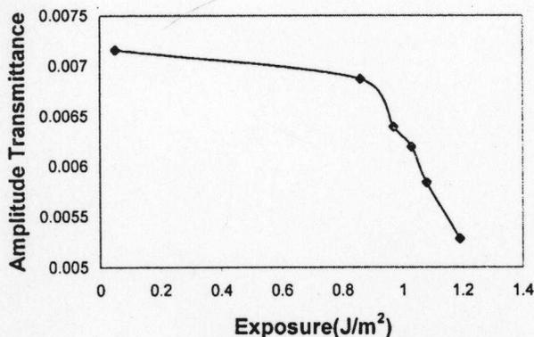
Fig. 9. Variation in the amplitude transmittance of the material as a function of exposure ( $J/m^2$ ).
