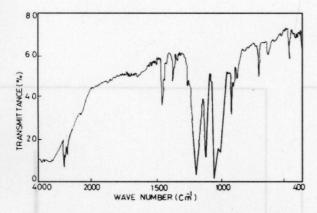
Figure 3 An IR spectrum of zinc butyl xanthate.
