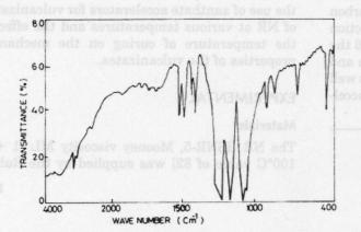
Figure 1 An IR spectrum of zinc ethyl xanthate.
