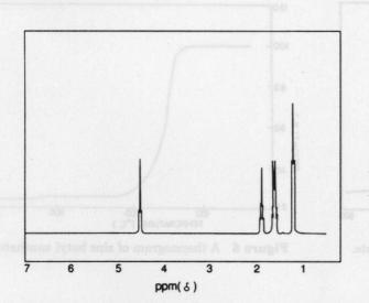
Figure 9 An H-NMR spectrum of zinc butyl xanthate.
