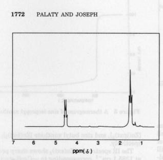
Figure 7 An H-NMR spectrum of zinc ethyl xanthate.
