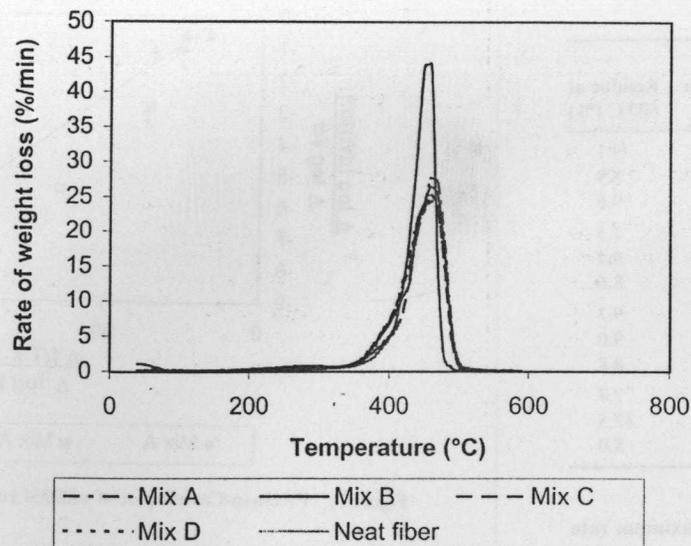
Figure 1. TGA traces of composites A-D.
