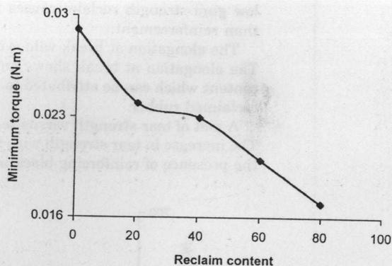
FIGURE 1 Variation of minimum torque with reclaim loading.
