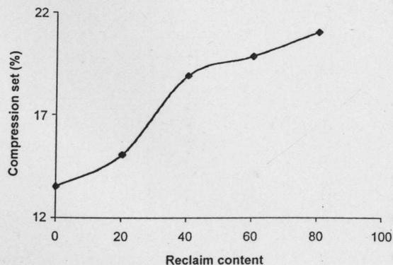
FIGURE 10 Variation of compression set with reclaim loading.
