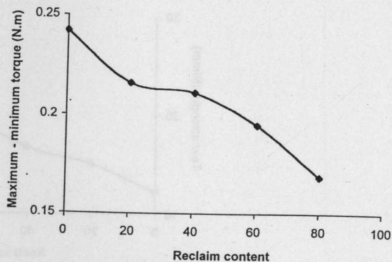
FIGURE 2 Variation of (maximum-minimum) torque with reclaim loading.
