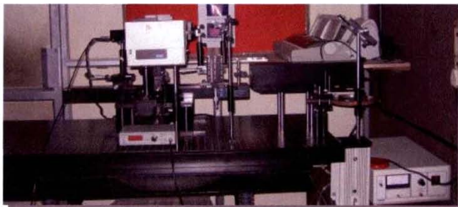
Fig. 1.4 Inbuilt PDS experimental setup mounted over a three arm unit with 150 W Xe-arc lamp (Oriell) as a broad band source. Monochromator (Oriell) seen in the foreground was used to separate the broad band into monochromatic beams that were used as the pump beam.
