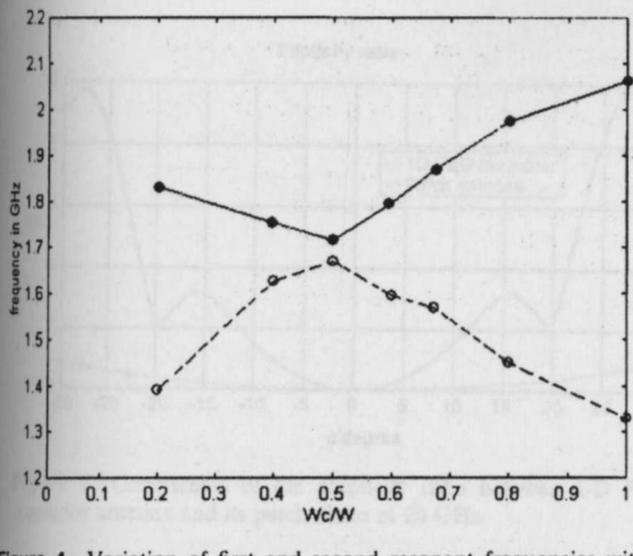
Figure 4 Variation of first and second resonant frequencies with central width. -○- first frequency, —●— second frequency
