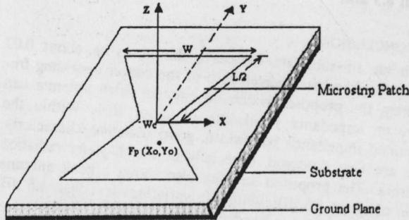
**Figure 1** Geometry of the proposed dual-frequency dual-polarized compact microstrip antenna
