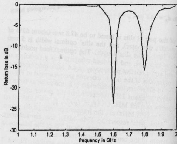
**Figure 2** Variation of return loss with frequency
