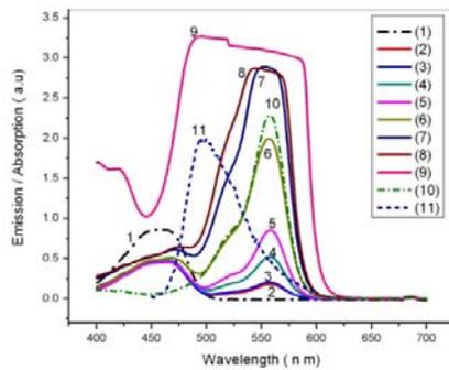
Fig. 2 Net absorption spectra of dye mixture doped PMMA rods along with pure donor emission. 1- [D] only ( $5 \times 10^{-5}$  m/l), 2- [A] =  $4 \times 10^{-5}$ , 3- [A] =  $7 \times 10^{-5}$ , 4- [A] =  $10^{-4}$ , 5- [A] =  $2 \times 10^{-4}$ , 6- [A] =  $4 \times 10^{-4}$ , 7- [A] =  $5 \times 10^{-4}$ , 8 - [A] =  $6 \times 10^{-4}$ , 9- [A] =  $7 \times 10^{-4}$ , 10- [A] ( $10^{-4}$  m/l) only, 11- donor emission
