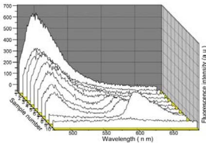
Fig. 3 The recorded fluorescence from dye mixture doped PMMA with 465 nm excitation.
