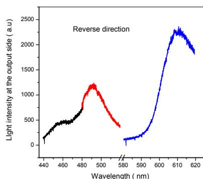
Fig.6 Transmission in the reverse direction.
