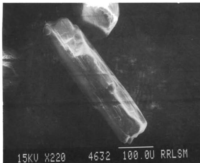
Plate 6b Estuarine sillimanite (+120 mesh). Note the well rounded terminals
