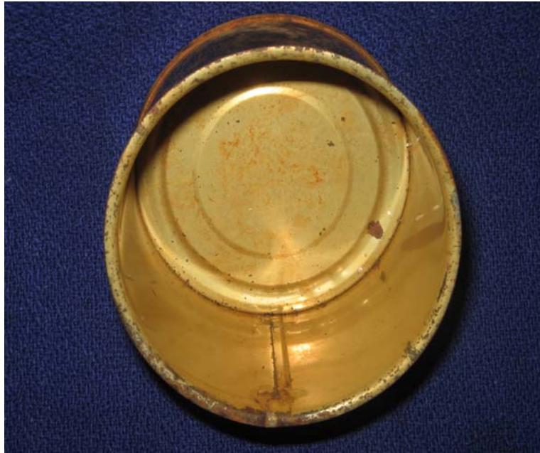
Plate-9 b. Lacquer failure in aluminium cans in the form of blisters and peel off
