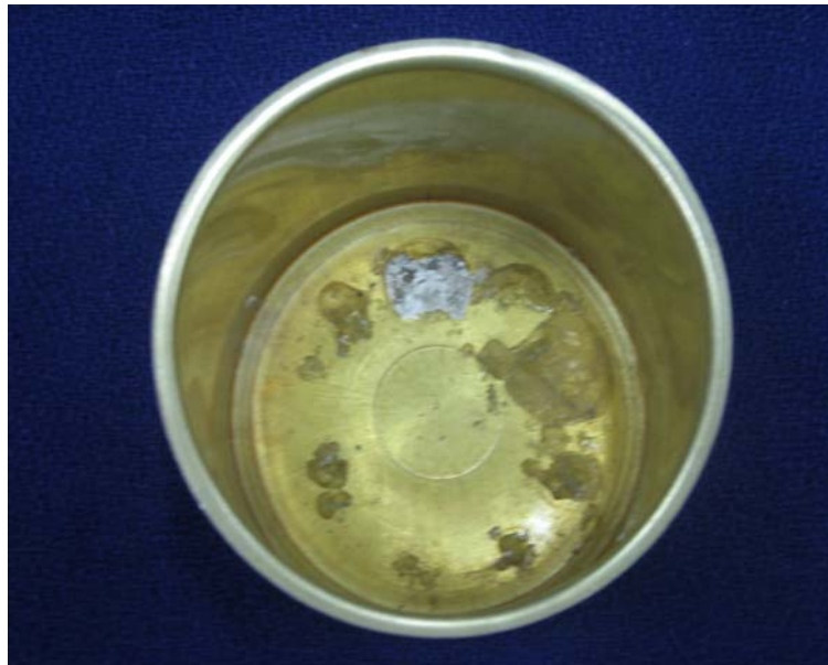
Plate-9 b. Lacquer failure in aluminium cans in the form of blisters and peel off
