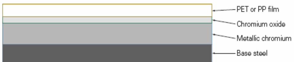
Plate-6 b. Functional layers of TFS can
