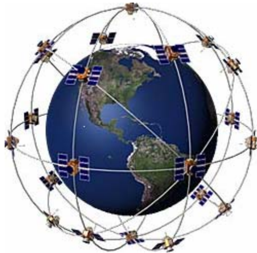
Figure 2.9: Schematic diagram of GPS constellation [Courtesy: NASA]
