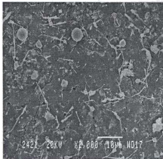
Figure 5.8 SEM micrograph showing typical surface morphology of CuInSe 2 thin film
