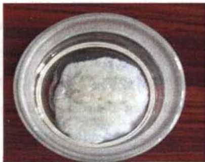
Figure 6.5. Result of solvent action on coagulum containing in situ precipitated silica.
