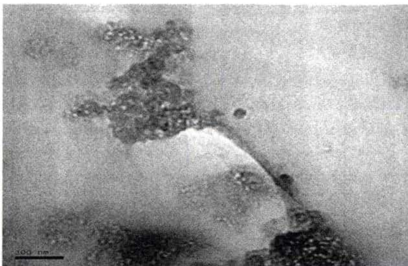
Figure 3.11a. TEM photograph of sample with 5phr silica
