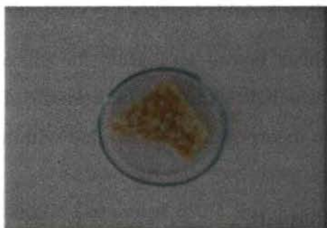
In situ precipitated silica sample before ignition
