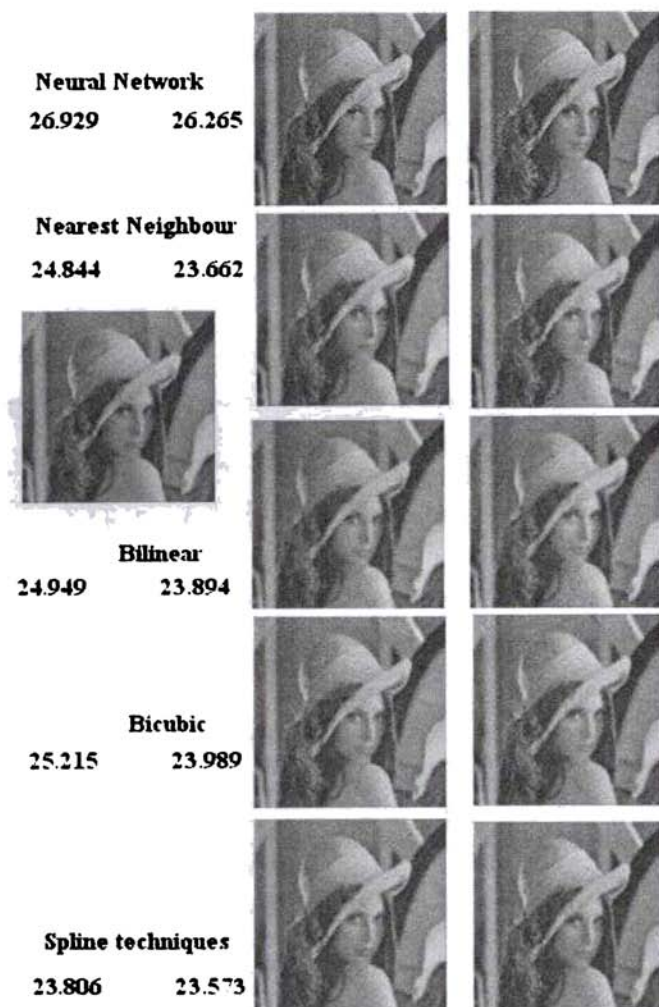
Fig. 5.15 Restoration of image using various interpolation techniques- a comparison 128 x 128 image is restored to 512 x 512 image with intermediate image of size 256 x 256
