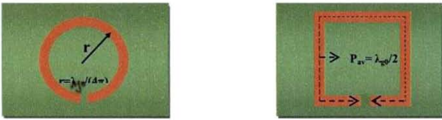
Fig. 1.5 Circular and square \lambda_{g0}/2 open loop resonators
