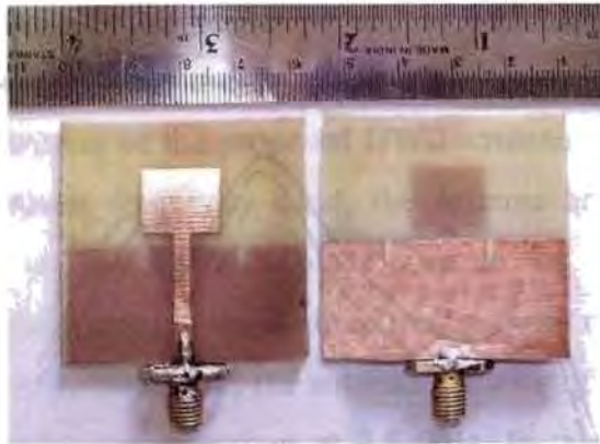
Fig.4.72 The top and bottom view of the prototype of optimized UWB rectangular monopole with slotted ground antenna W_g=45\text{mm} , L_g=18\text{mm} , d=2\text{mm} , S_w=14\text{mm} , S_l=10\text{mm} , 'x' = 1mm, 'y' = 3mm, 'Vx' = 18mm, h=1.6\text{mm} , \epsilon_r=4.38 Overall size (30 \times 45)\text{mm}^2 .
