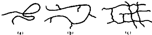
Fig.1.3. Schematic Representation of Polymer Molecules: (a) Linear (b) Branched (c) Cross-linked
