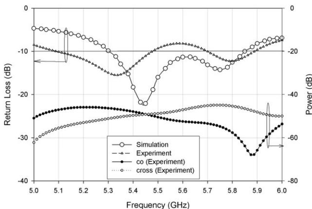
**Figure 3** Measured return loss, co and cross powers with  $L = 36$  mm,  $L_1 = 23$  mm,  $L_2 = 23$  mm, and  $L_3 = 3$  mm,  $\epsilon_r = 4.4$  mm,  $h = 1.6$  mm, and  $Wt = 3$  mm
