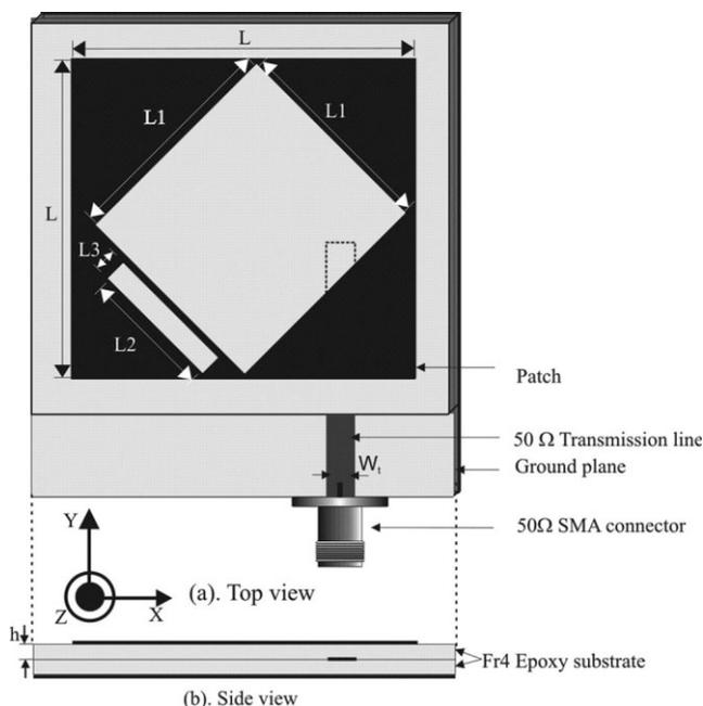
Figure 1 Antenna Geometry
