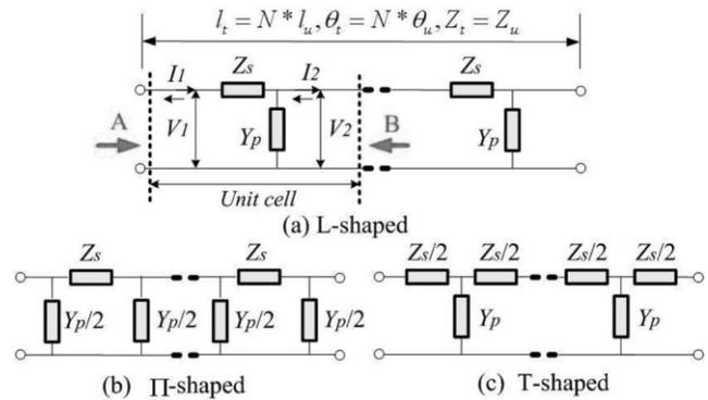
**Figure 1** Three types of general periodical circuit models with L-shaped, II-shaped, and T-shaped
