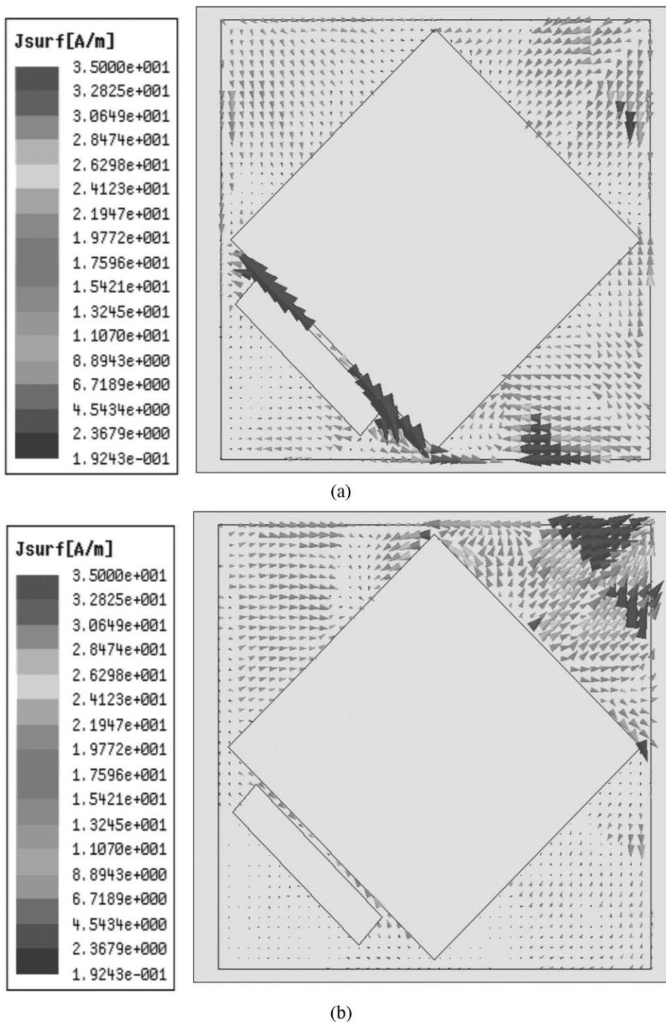
**Figure 5** (A) Simulated surface current distribution of the proposed antenna at  $f = 5.3$  GHz. (b) Simulated surface current distribution of the proposed antenna at 5.8 GHz
