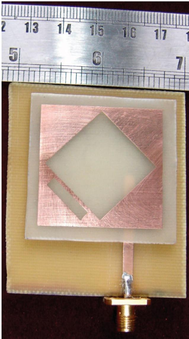
**Figure 2** Photograph of the proposed antenna. [Color figure can be viewed in the online issue, which is available at [www.interscience.wiley.com](http://www.interscience.wiley.com)]
