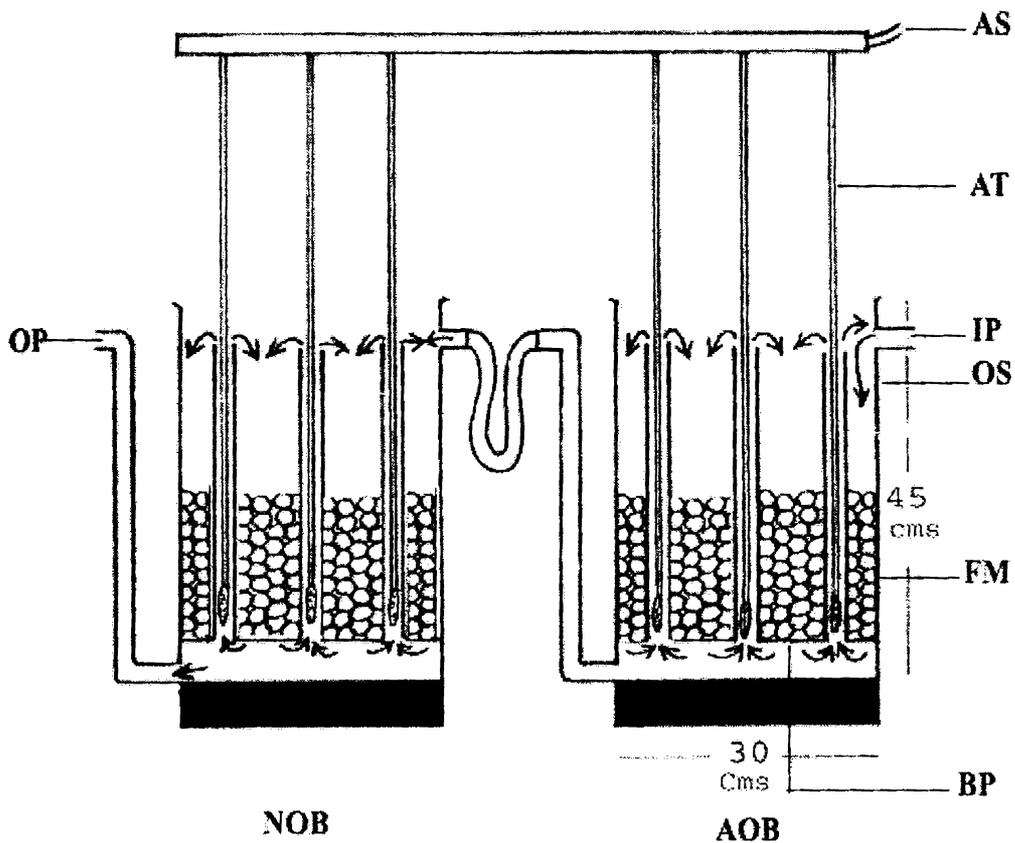
**Fig.1.** Cross sectional view of the bioreactors connected serially
