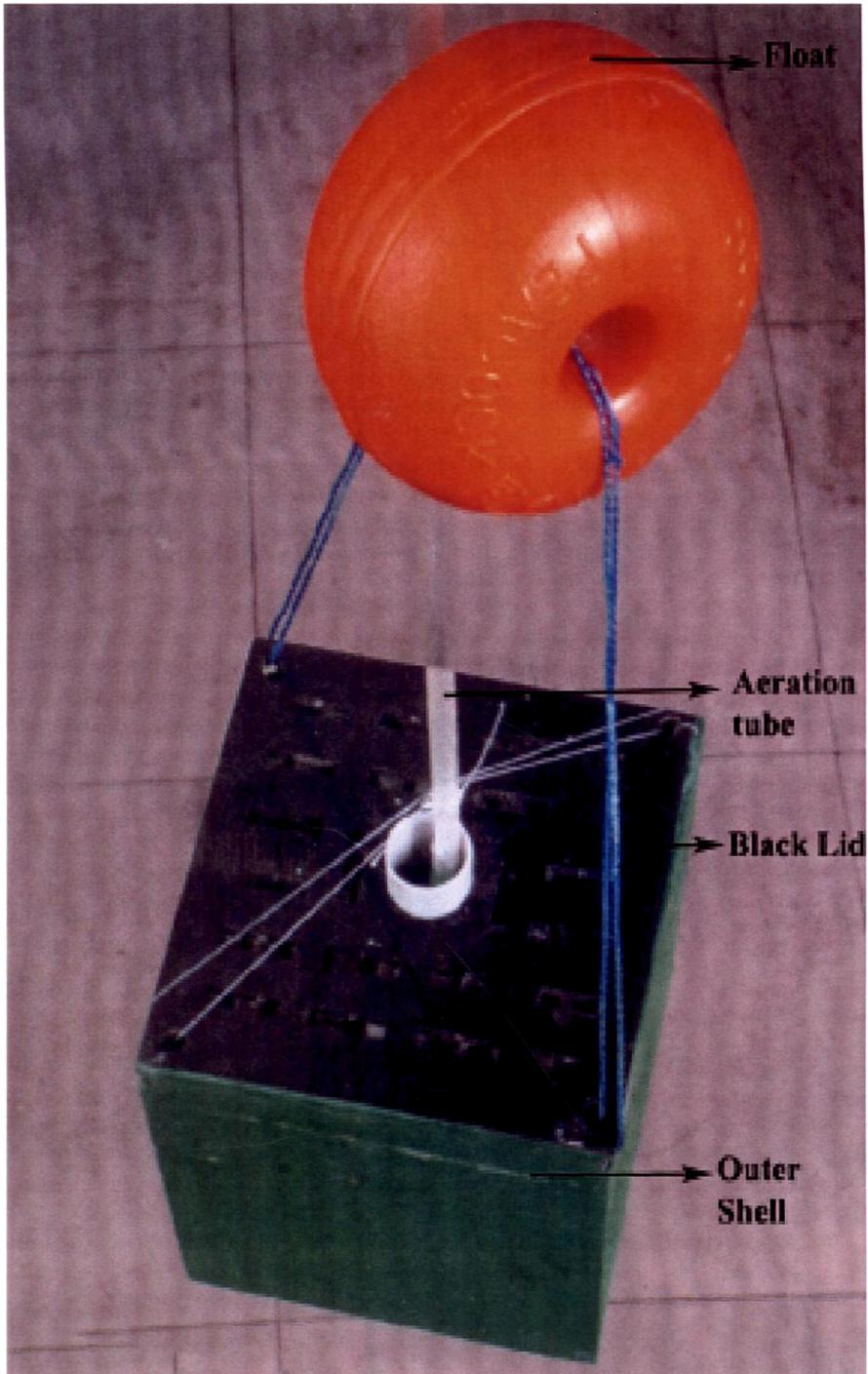
**Fig.4.** Stringed Bed Suspended Bioreactor on full assembly (SBSBR)
