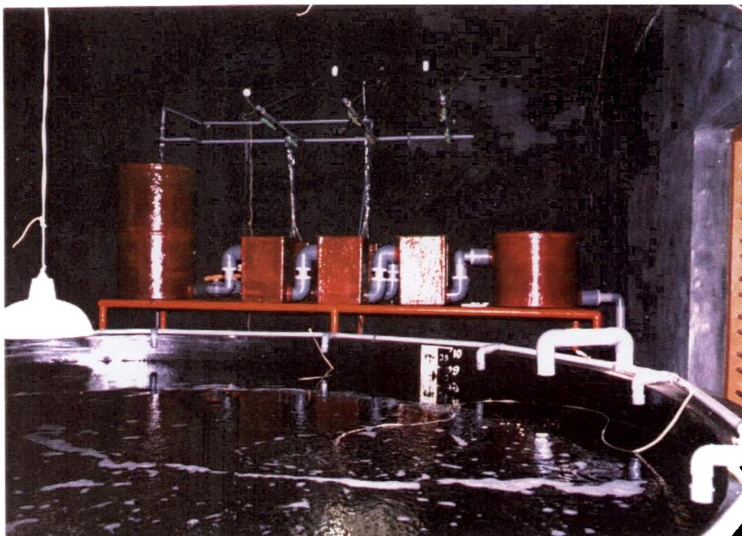
**Fig.2.** A fully assembled Packed Bed Bioreactor (PBBR) System
