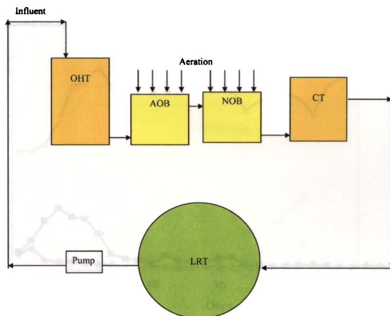
**Fig. 1.** Process flow diagram of the reactors integrated into the larval rearing tank (OHT-overhead tank with automatic water level controller, AOB-ammonia oxidizing bioreactor, NOB-nitrite oxidizing bioreactor, CT-collection tank for the treated water, LRT- larval rearing tank)
