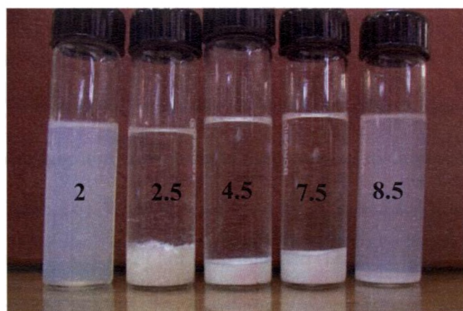
Figure 2.5. Photograph of the titania nanoparticles peptised at different pH (i) 2 (ii) 2.5 (iii) 4.5 (iv) 7.5 (v) 8.5
