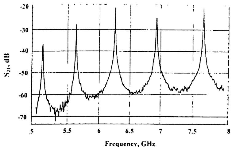
FIGURE 2b: Resonant frequency spectrum of J-band cavity resonator.
