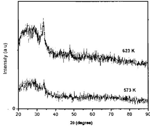
Figure 6.1: XRD patterns of the as-prepared cerium oxide thin films at 573 K and 623 K.
