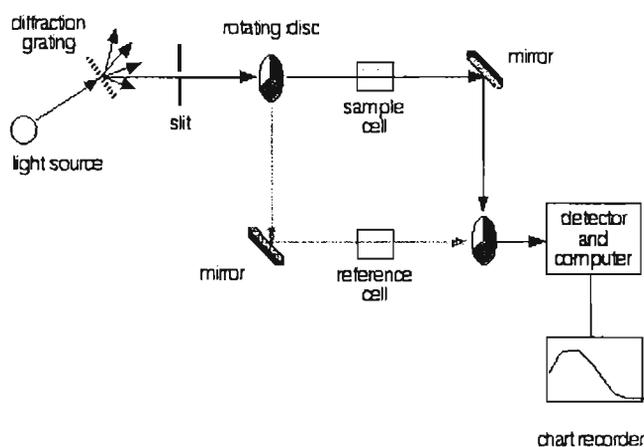
Figure.2.5: Double beam UV-visible spectrometer
