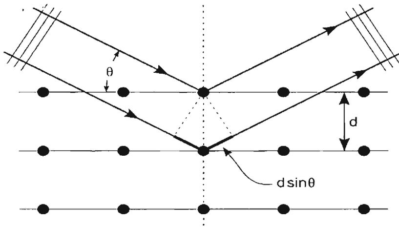
**Figure 2.2:** X-ray diffraction from crystal planes.
