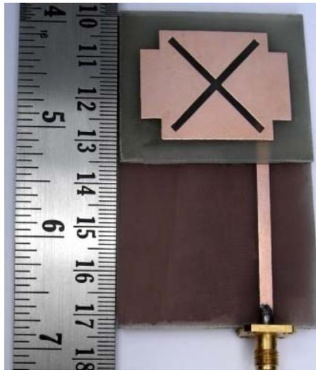
**Figure 3.14** Prototype of the fabricated dual-frequency dual-polarized cross patch antenna with X-slot ( $L=30.9\text{mm}$ ,  $W=43.5$ ,  $L_s=5.1$ ,  $L_x=18.3$ ,  $W_x=2.3$ ,  $L_g=W_g=75$ ,  $W_{\text{off}}=6.8$ ,  $h=1.6$  (All are in mm)  $\epsilon_r=4.4$ )
