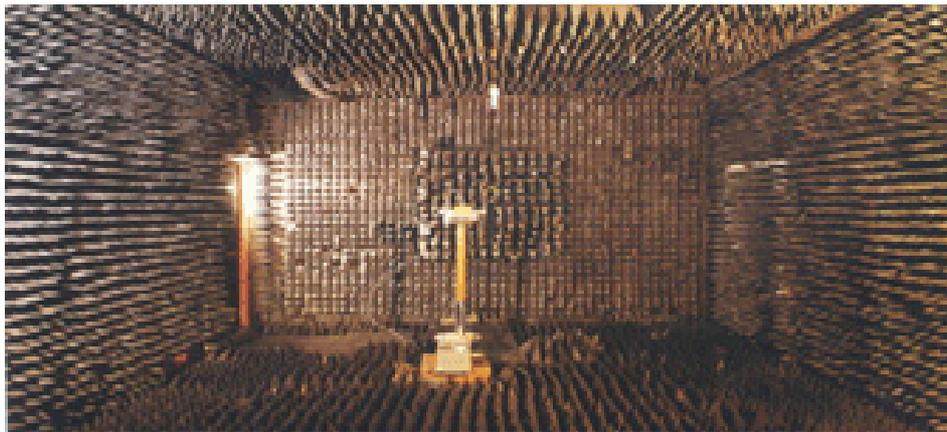
**Figure 2.3** Photograph of the anechoic chamber used for the antenna measurements
