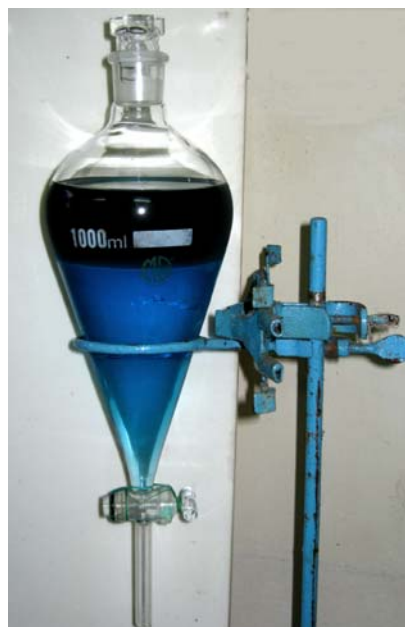
Fig. 2 Phase separation of pyocyanin to form a blue pyocyanin-chloroform lower layer and an upper aqueous layer.
