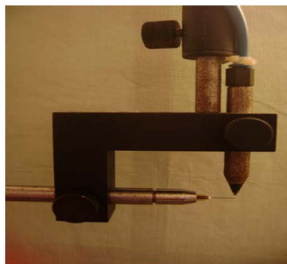
Figure 2.2: Photograph of the air blast type spray nozzle used for the work.
