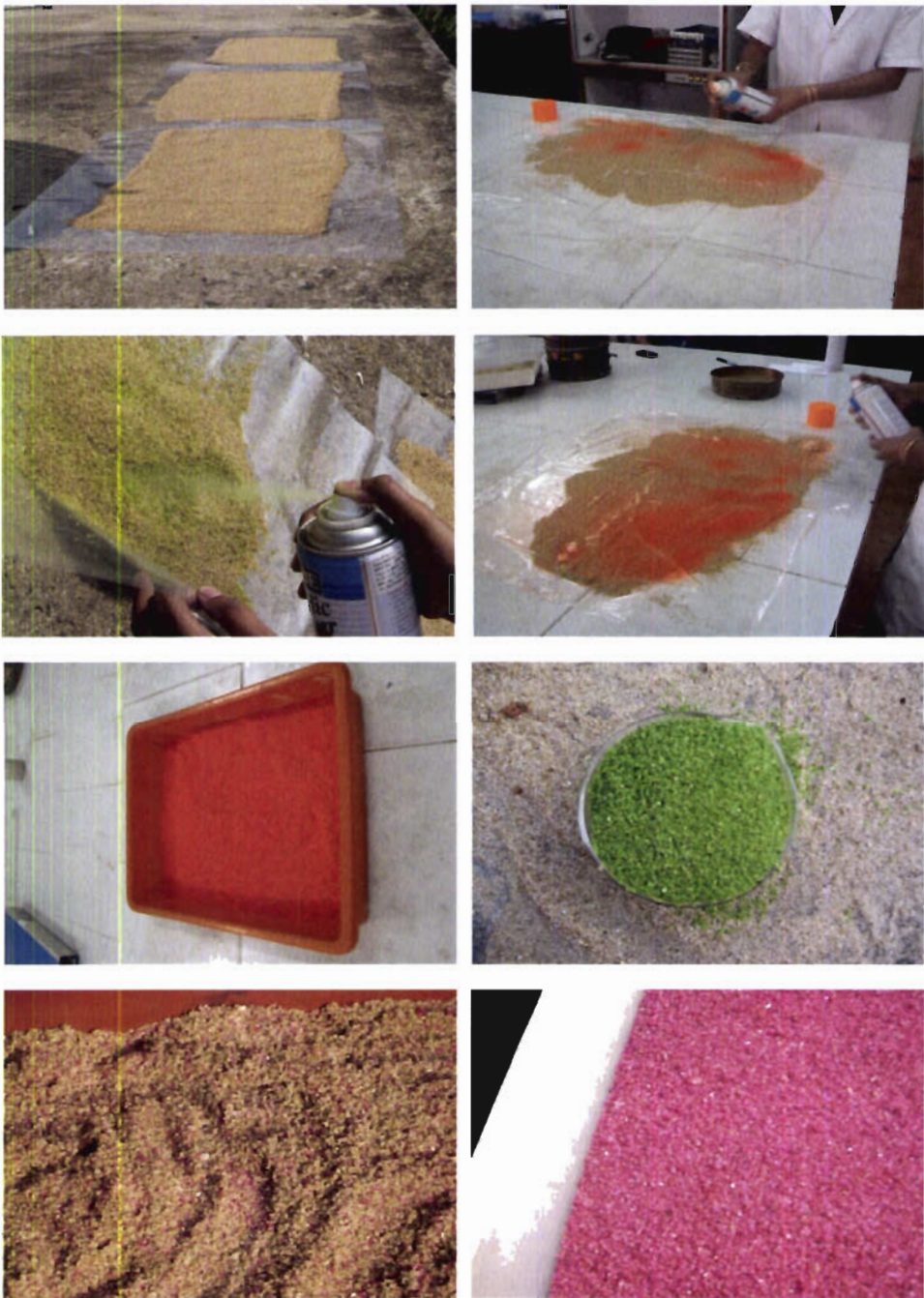
Preparation of fluorescent tracer particles
