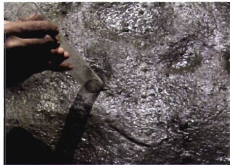
Collecting sediment core samples from experimental tanks
