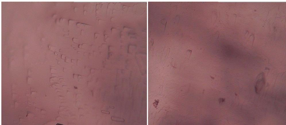
**Fig: 5.9** Etch patterns of (a) CKDP (b) LKDP
