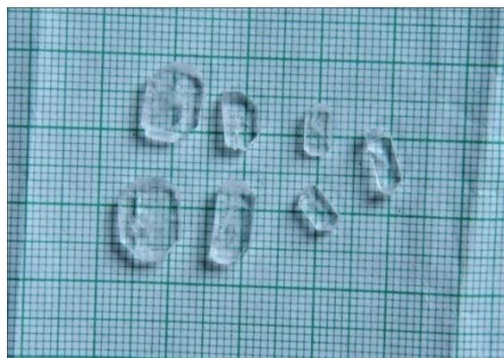
**Fig: 5.1(b)** Photographs of L-lysine doped KDP crystals
