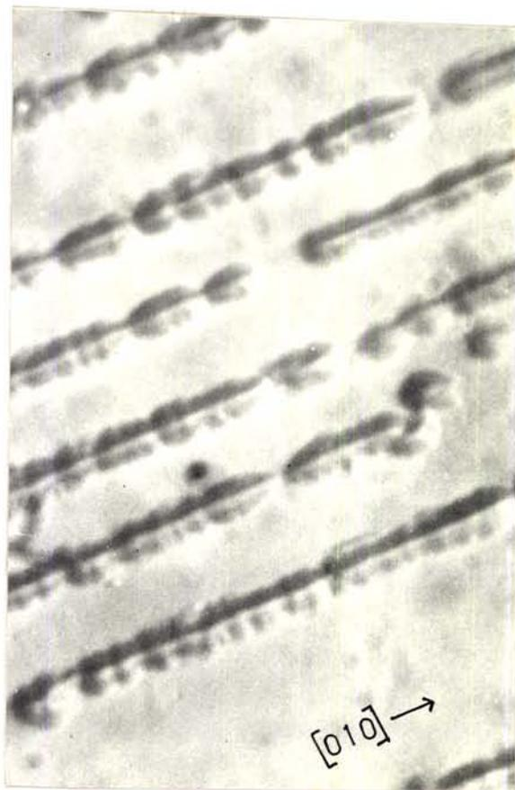
Fig.6.11 Array of pits along  $[010]$  direction on (001) face of DAHC. ( $\times 360$ )
