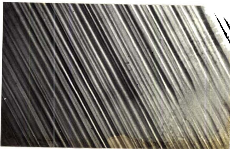
Fig.6.13 Slip lines on (001) surface of DAHC. Etching time 30 secs. (x500)
