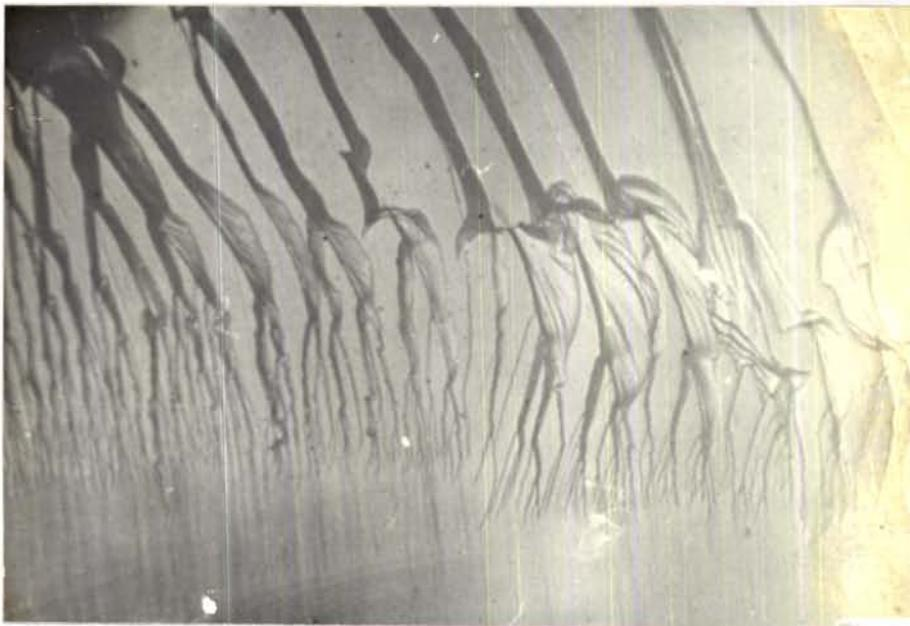
Fig.8.3 A river pattern observed on the cleavage face of DAHC. (x160)
