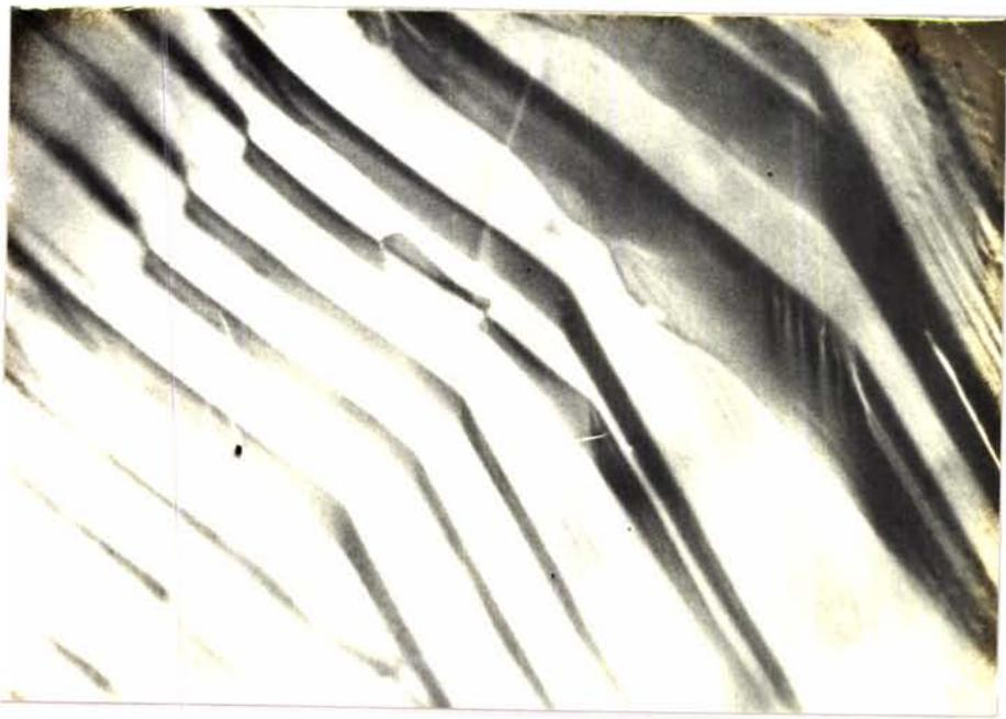
Fig.8.11 Rectilinear markings showing instances of rectilinear cleavage. (x600)
