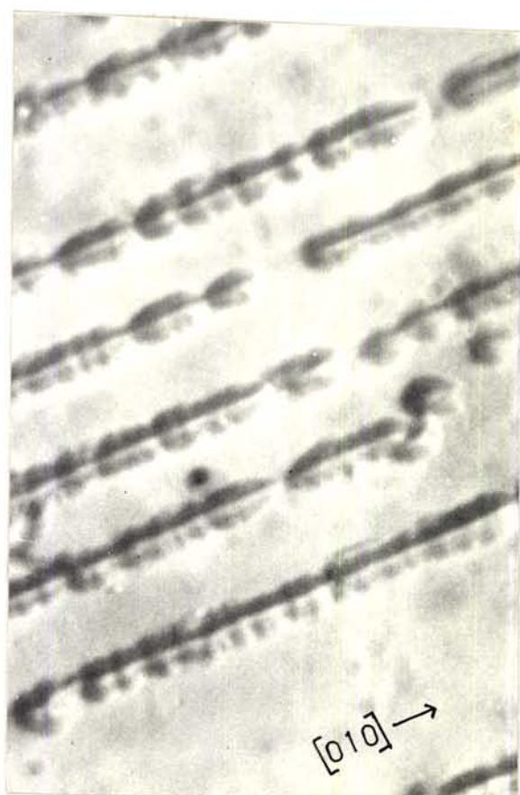
Fig.6.11 Array of pits along  $[010]$  direction on (001) face of DAHC. ( $\times 360$ )
