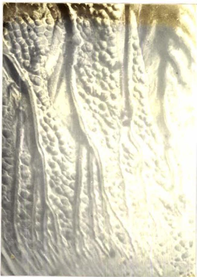
Fig.8.6 An etched cleavage surface containing river patterns. (x200)
