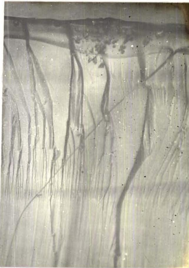
Fig.8.4 Micrograph showing rivulets which merge with a large step that run perpendicular to them. (x100)
