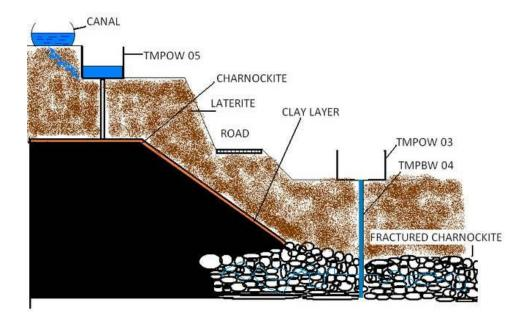
Figure 6.1 Schematic representation of Dug-cum-Bore wells (TMPOW-03, TMPBW-04 and TMPOW-05)
