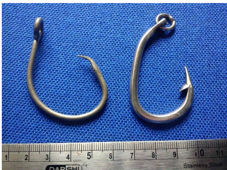
Fig. 6.1 Hooks used for the study - 14/0 Circle hook (left) and 3.5 Japanese tuna hook (right)
