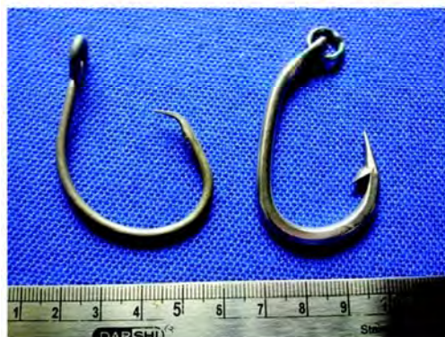
Fig. 1. Hooks used for the study- 14/0 circle hook (left) and 3.5 Japanese tuna hook (right)
