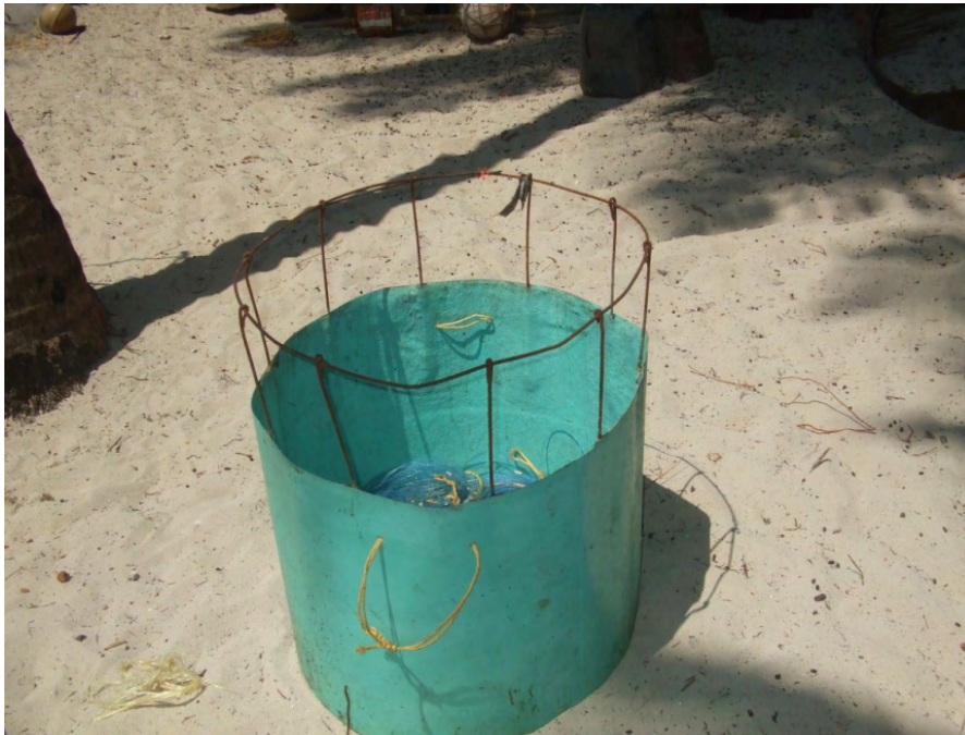
Fig. 3.14 FRP bin for storing branchlines
