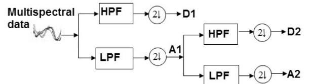
Fig. 2. Wavelet Analysis of multispectral data
