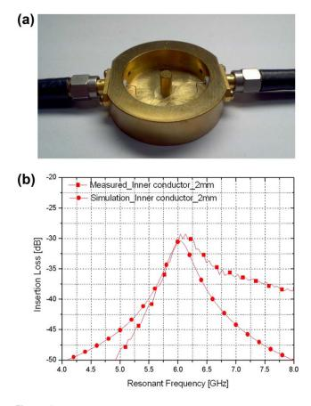
**Figure 8** Fabricated resonator with a = 2 mm, b = 14 mm, l = 8.5 mm, and measured insertion loss. (a) Fabricated resonator and (b) insertion loss. [Color figure can be viewed in the online issue, which is available at wileyonlinelibrary.com]
