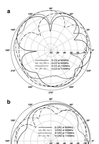
**Figure 7** Measured (a) copolar radiation pattern and (b) cross polar radiation pattern at two different frequencies (1) 900 MHz and (2) 1.15 GHz
