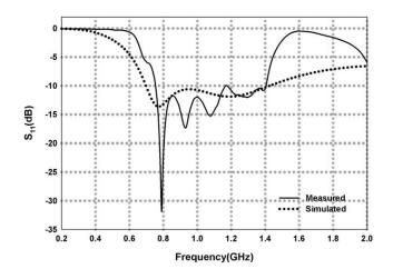
Figure 2 Reflection coefficient of the proposed antenna
