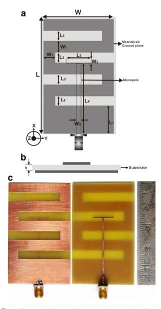
**Figure 1** (a, b) Geometry of the proposed antenna (L = 50 mm, W = 30 mm,  $L_1 = 12$  mm,  $L_2 = 4$  mm,  $L_3 = 4.2$  mm,  $L_4 = 31.5$  mm,  $L_5 = 10$  mm,  $W_1 = 5$  mm,  $W_2 = 0.6$  mm, h = 1.6 mm,  $\varepsilon_r = 4.4$ ) and (c) Photograph of the proposed compact antenna. [Color figure can be viewed in the online issue, which is available at wileyonlinelibrary.com]
