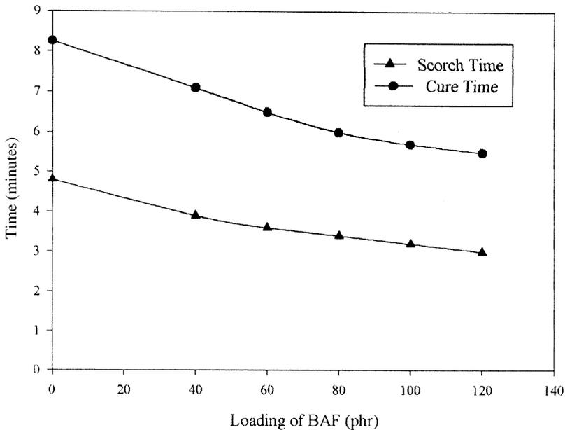
**FIGURE 1** Scorch time and cure time versus loading of fillers.
