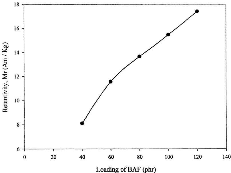
**FIGURE 5** Retentivity versus loading of fillers.
