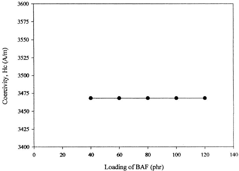
**FIGURE 6** Coercivity versus loading of fillers.
