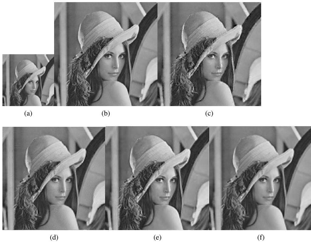
Figure 3.28: (a)Low resolution image (b)Original image (c)Freeman method(d)wavelet method 1(e) Sapan's wavelet method (f)block wavelet method
