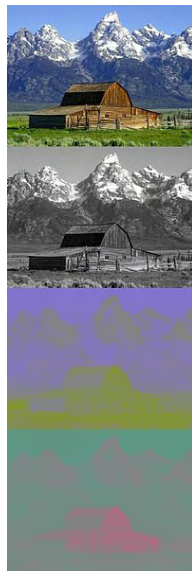
Figure 6.5: A color image and its Y , C_b and C_r components.
