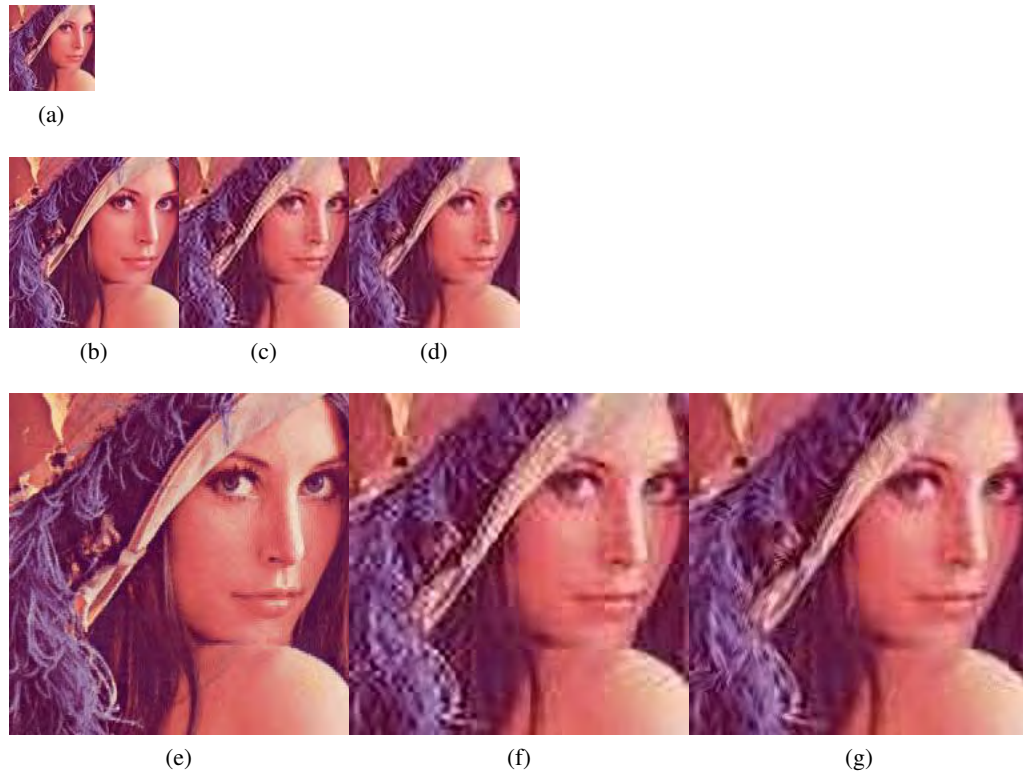
Figure 6.14: (a)low resolution image(64x64)(b)original image(128x128)(e)original image(256x256) (c),(d)2 times SR images (128x128) using Yang et al method and directionlet method (f),(g) 4 times SR images (256x256) using Yang et al method and new directionlet method respectively.
