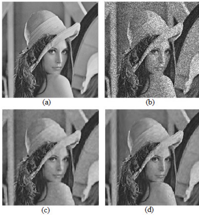
Figure 5.23 Despeckling result for synthetic speckle image of Lena (four-look amplitude). (a) Original Lena image (b) Speckled Lena image. (c) Despeckled image using GGMAP-S algorithm. (d) Despeckled image using DT-CG
