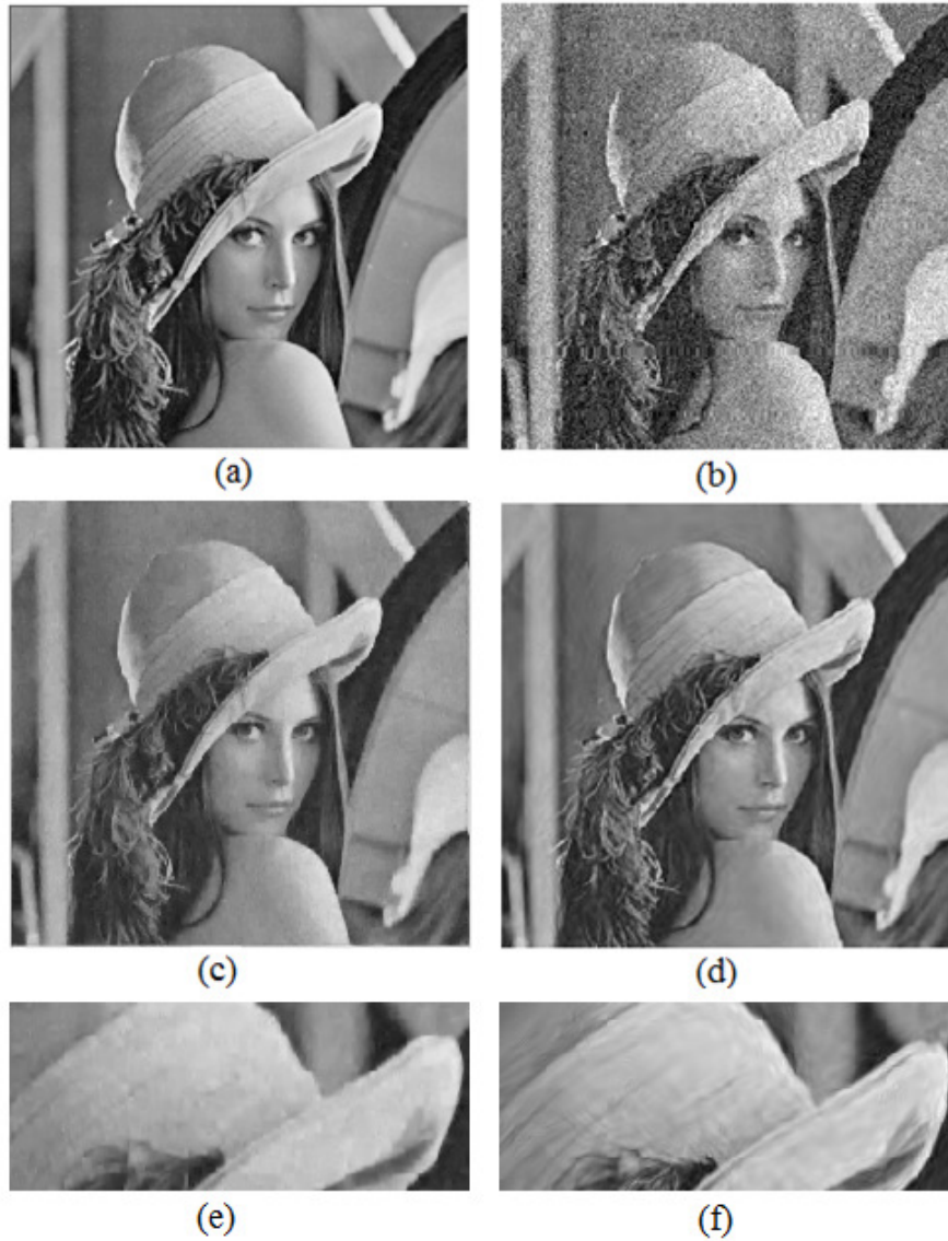
Figure.4.3. Image denoising result of Lena image. (a) Noise free image (b) noisy image with \sigma = 20 , (c) denoised image using WT-SURE (d) denoised image using DT-SURE (e) enlarged portion of (c) and (f) enlarged portion of (d)
