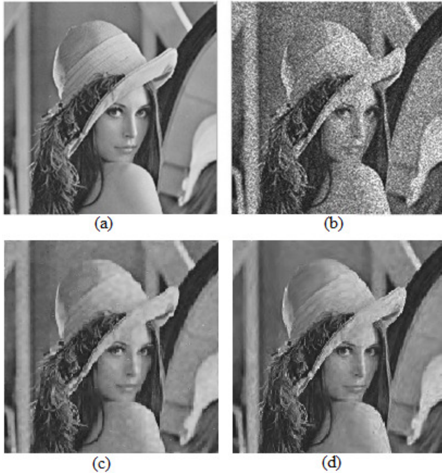
Figure 5.17 Despeckling result for synthetic speckle image of Lena (four-look amplitude). (a) Original Lena image (b) Speckled Lena image (c) Despeckled image using wavelet based LGMAP-S (d) Despeckled image using DT-LG scheme.
