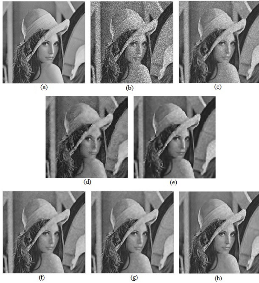
Figure 5.27 Despeckling results of Synthetic SAR image of Lena in amplitude format with L=4 (a) Original noise free Image (b) Noisy image (c) Despeckled image using Lee filter (d) Despeckled image using NSCT (e) Despeckled image using NSST and (f) Despeckled image LGMAP-S (g) Despeckled image GGMAP-S (h) Despeckled image DT-Bivariate
