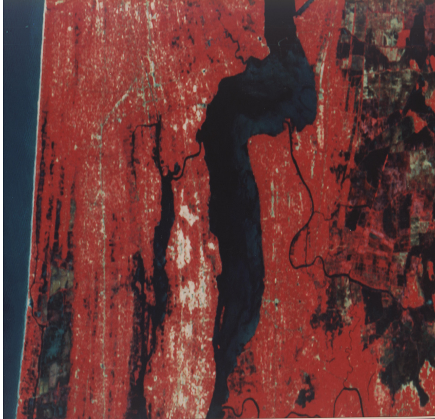
Fig. 2.20. Geocoded image showing strand lines along the coast
