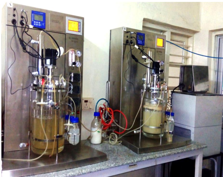
**Fig. 5.2:** Production of *Bacillus* MCCB 242 phytase in 5L bench top laboratory scale fermentor
